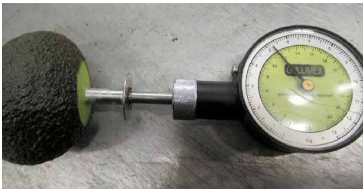
Figure 37 — Photo of Penetrometer
