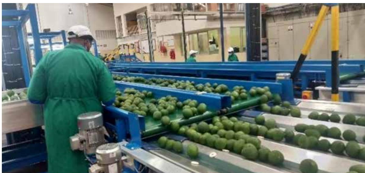
Figure 41 — Sorting of Avocado along the grading line in a packhouse
